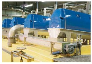
Roto-Sieve drum screens, model RS-51, installed at Kullavik treatment works in Kungsbacka.
